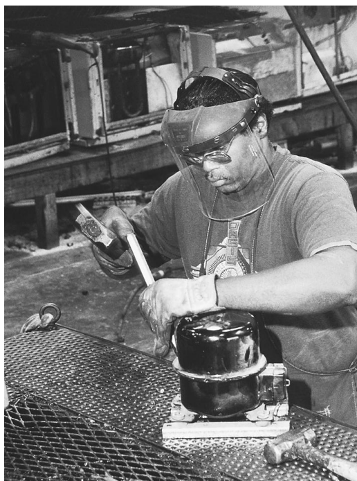
THIS WORKER IS REMOVING FREON FROM AN OLD REFRIGERATOR. CFCs LIKE FREON MAY BE RESPONSIBLE FOR THE DEPLETION OF THE OZONE LAYER. (James A. Sugar/Corbis. Reproduced by permission.)
